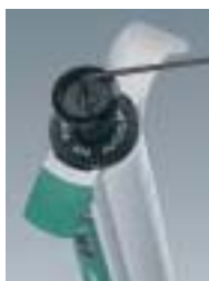
Calibration screw located under comfort pad of plunger button. (Key supplied with instrument.)
