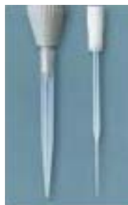
Use of a glass Pasteur pipette with the adaptor supplied, even when protection filter installed.
